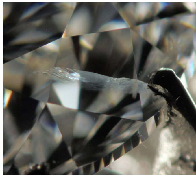
Figure 6: A fissure, observed in the same synthetic diamond that is similar to those found in a natural diamond.
