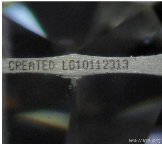
Figure 16: Laser inscription on a CVD synthetic diamond manufactured by Gemesis.
