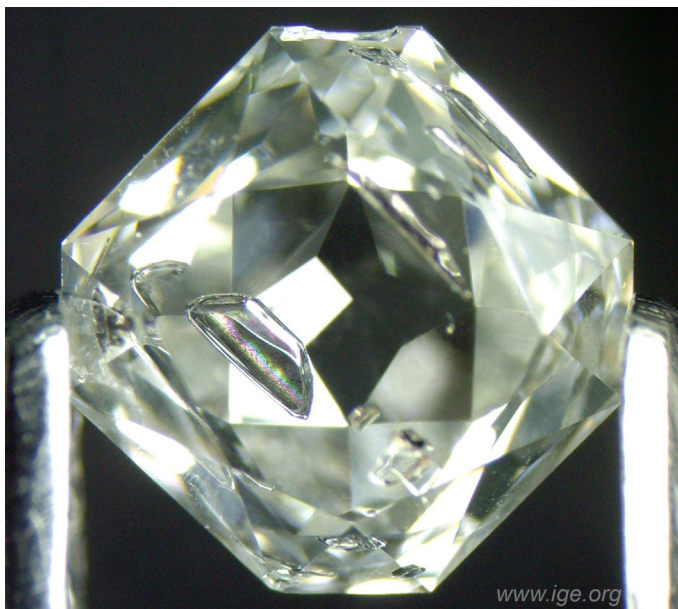
Figure 1: Large metallic inclusions with iridescent patina on a colorless HPHT synthetic diamond.
