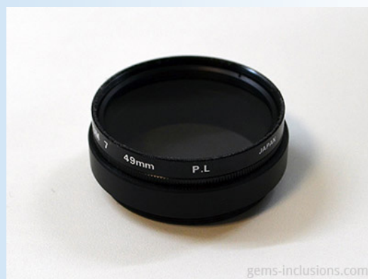
Plane-polarizing filter with additional adapter ring for mounting on microscope.
