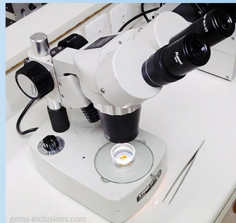
The simplest way to observe a gemstone in immersion, using a standard vertical microscope and glass cell and moving the stone with a pair of tweezers. (IGE)
