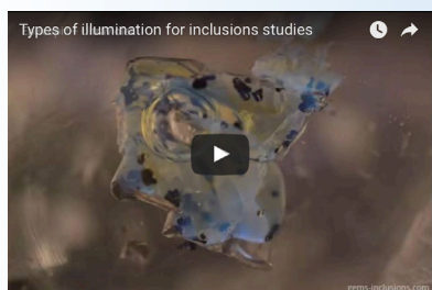
Same fluid inclusion recorded in transmitted, episcopic and ultraviolet illumination.
