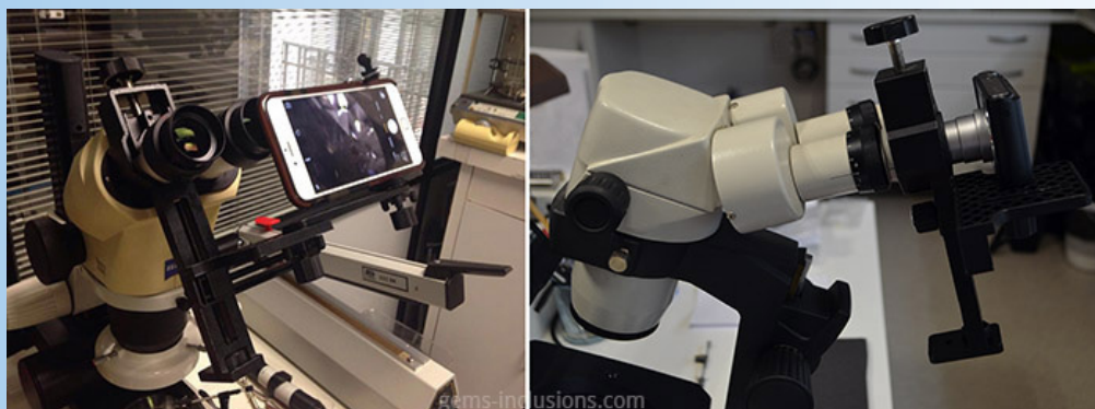
Digiscoping adapter used with smartphone (left: Lozano Gemologos) and with compact digital camera (right: IGE)
