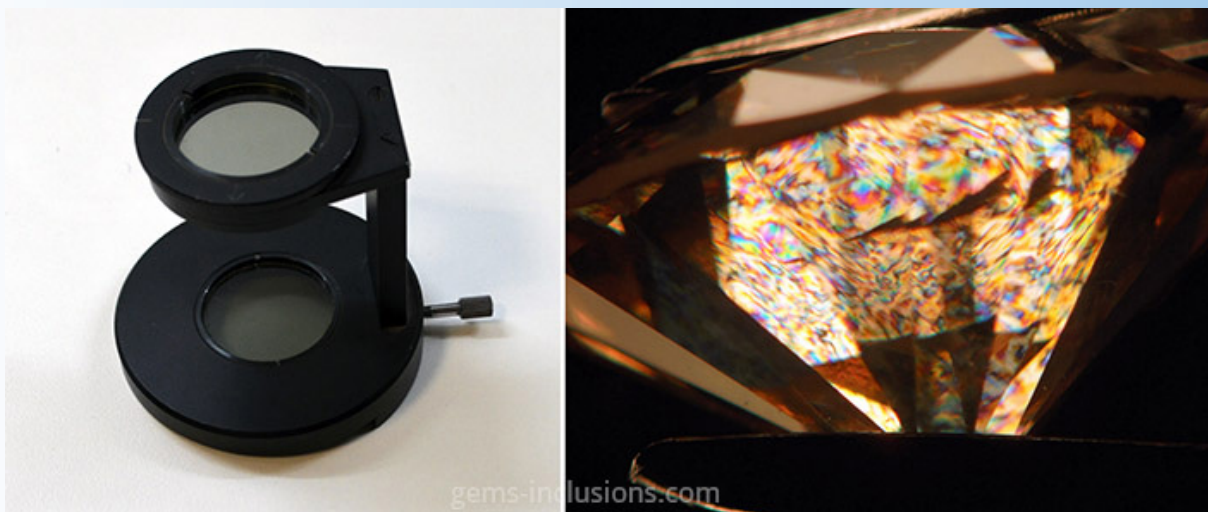
A pair of crossed polars to use with a microscope (left) and anomalous birefringence in natural type Ia diamond (right). Field of view 6 mm.
