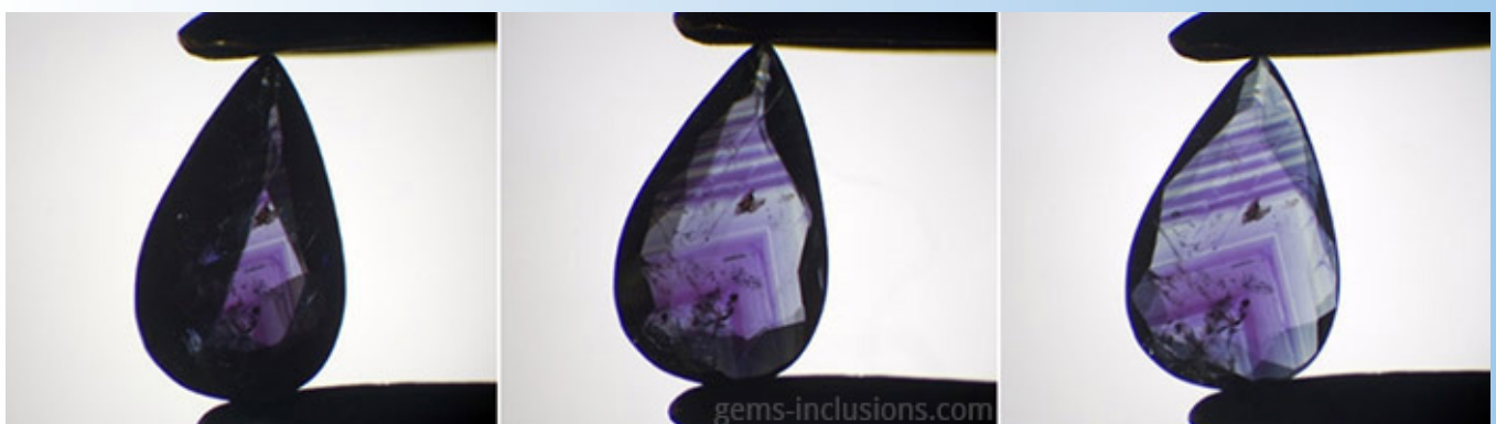
Same stone (Natural Brazilian Alexandrite, RI 1.67, 0.11 ct) observed in air (left) and in two different immersion liquids: alcohol (center) and toluene (right).
