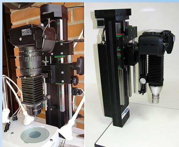
Left: Camera with extension rings, accordion bellows and Schneider Componon lens on Macrorail stage. Right: Camera with accordion bellow and microscope objective (Macrorail.com)
