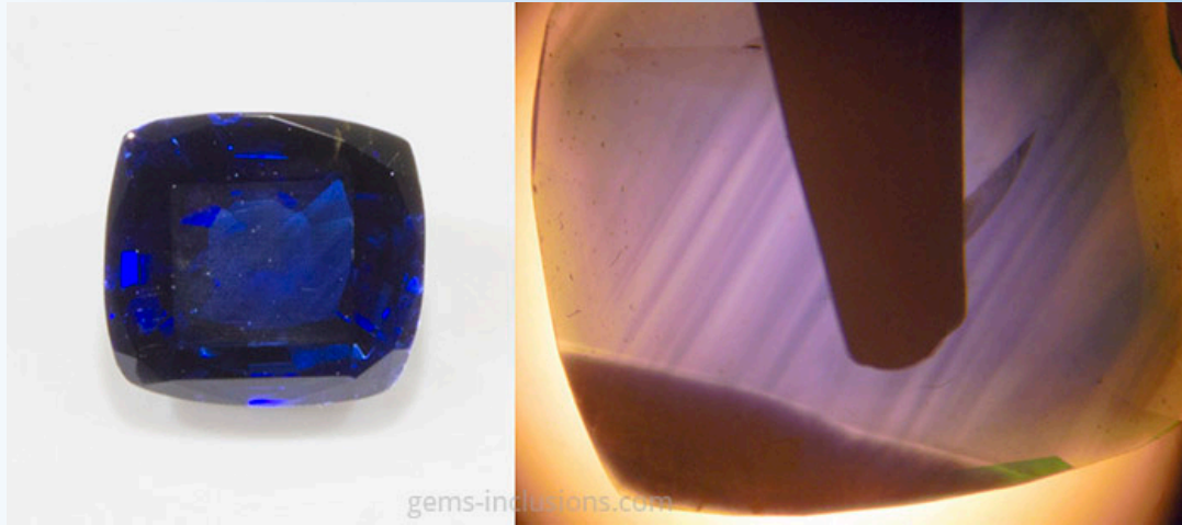
Natural sapphire observed in air and in methylene iodide immersion. Straight color zoning, typical for natural sapphires, is only visible in immersion.
