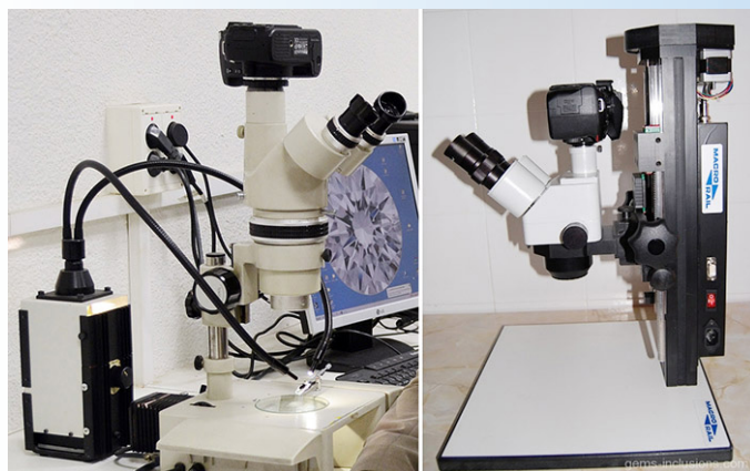
Digital reflex cameras mounted on different trinocular microscopes. Left: Nikon SMZ 10 (IGE) Right: B & Crown Head on Macrorail stage.
