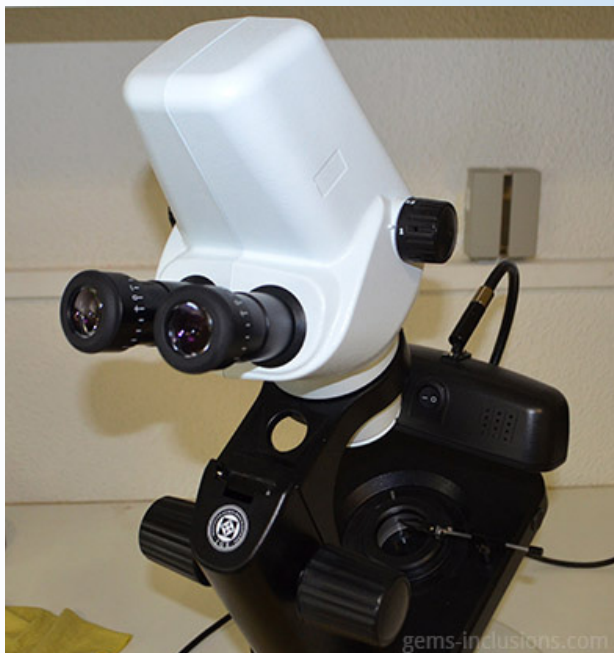
Gemmological Microscope BestScope with Digital Camera incorporated in Microscope's head (IGE)
