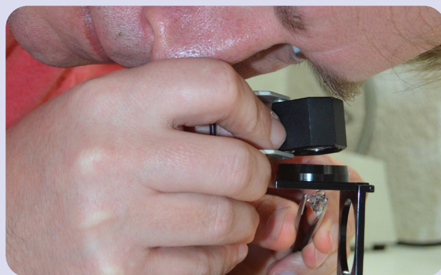
Figure 2a: Observation of anomalous birefringence in a diamond in a compact polariscope. The stone is held between its table and culet in tweezers and placed between cross polarizers, where it is observed with the 10x loupe, rotating the stone to see the interference figures in different directions (IGE).
