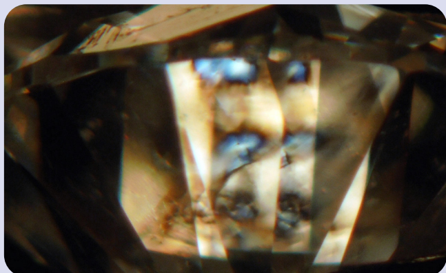
Figure 2c: Typical interference figures for a natural type Ia diamond, anomalous birefringence pattern mottled with second order interference colors. This pattern rules out the possibility that the diamond is synthetic HPHT or CVD (IGE).
