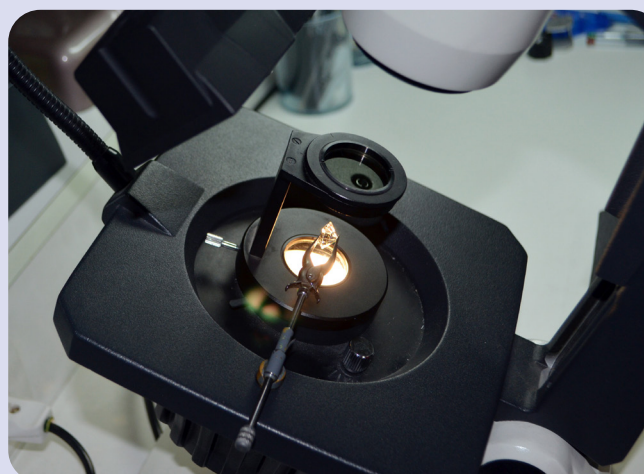
Figure 2b: The same test is performed much better on a gemological microscope with cross polarizers (IGE).
