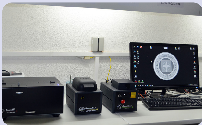
Figure 5c: The FTIR, UV-Vis-NIR and Raman-PL spectrometers from M & A Gemmological Instruments at the IGE Laboratory (IGE).
