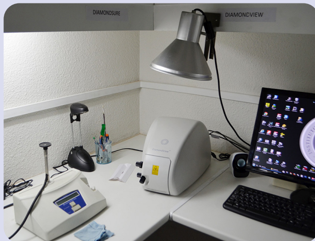
Figure 5a: The DiamondSure (left) and DiamondView (right) by De Beers at the IGE Laboratory (IGE).
