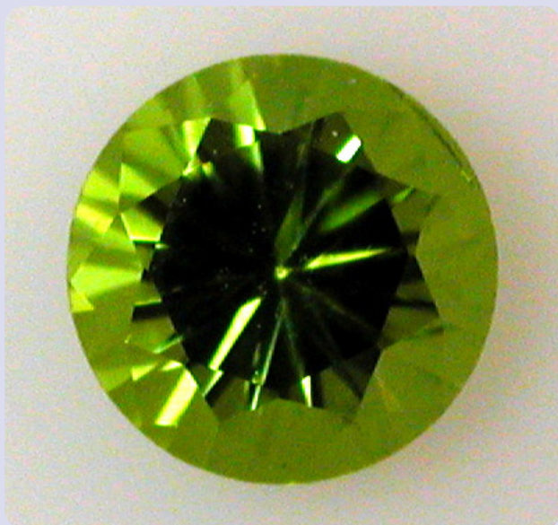
Figure 12. Round brilliant cut peridot with 45° pavilion retroreflecting the dark camera lens causing its dark table nail head appearance.
