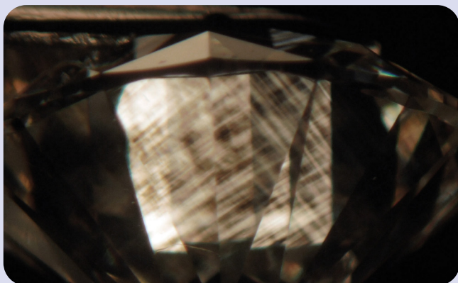
Figure 3a: Anomalous birefringence pattern ‘tatami’, typical for CVD synthetic diamonds and also for natural type II (IGE).
