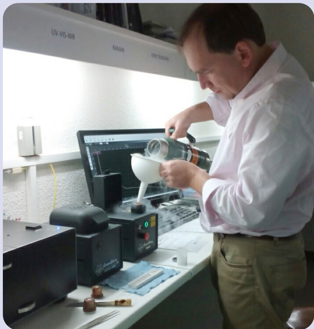
Figure 5d: For better observation of photoluminescence spectra in diamonds, liquid nitrogen is used to cool the sample (IGE).
