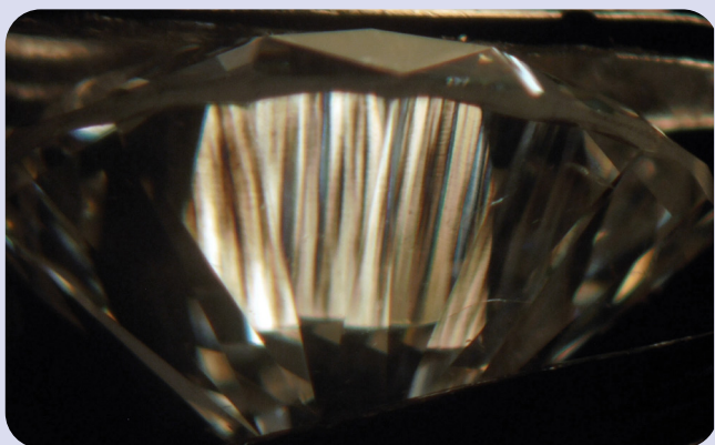
Figure 3b: Anomalous ‘columnar’ birefringence pattern, observed in some directions on CVD synthetic diamonds. In other directions the same diamond has the ‘tatami’ pattern (IGE).
