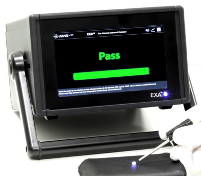
Figure 1. EXA working in 'Basic' mode, with 'PASS' result on the screen corresponding to natural diamond.
