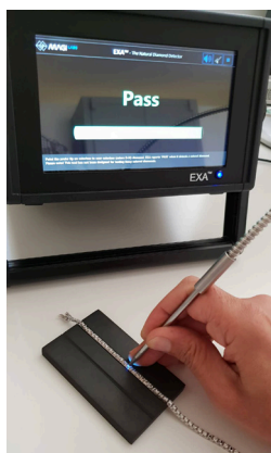
Figure 10. Checking small natural diamonds set in jewelry becomes a very easy task with EXA.
