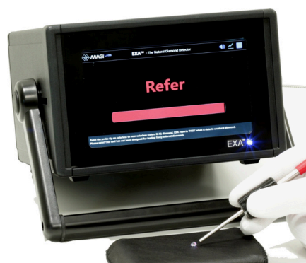
Figure 2. 'REFER' reading in 'Basic' mode corresponds to synthetic diamonds, imitations and a very low percentage of natural diamonds. 'REFER' stones will need additional testing to be identified; however, some of them can be positively identified in 'Advanced' mode.
