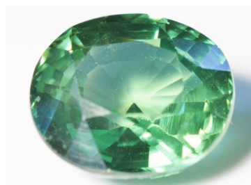
Synthetic Corundum Colored by Chromium & Nickel
