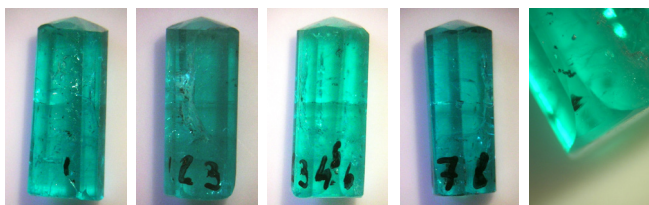
Figure 3: An unnatural number of faces were seen: seven faces (1,2,3,4,6,7,8) plus a small one (5) (3rd image from the left).
