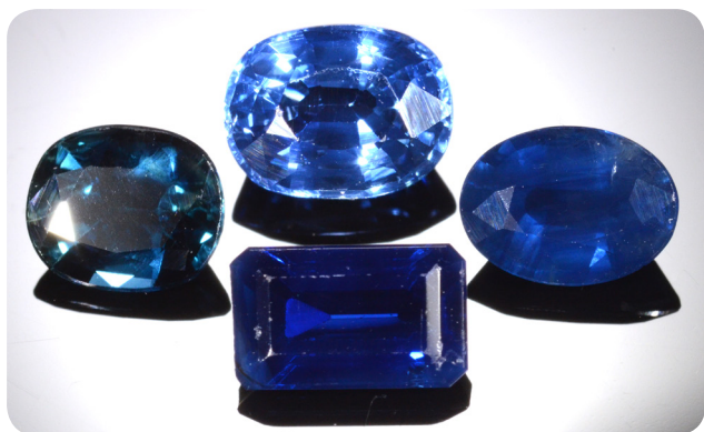
Figure 7: Four natural sapphires chosen to compare their properties to the example synthetic gems. Each exhibited no fluorescence response under SWUV illumination indicative of their natural origin.
