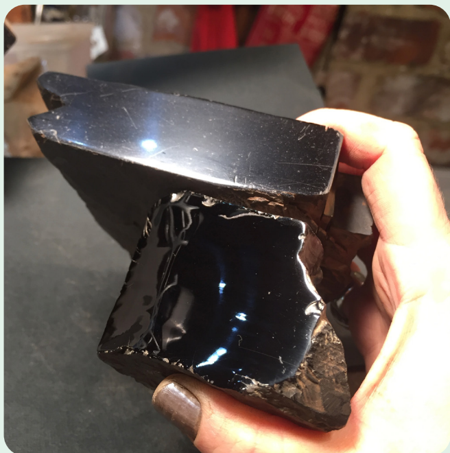
Very distinct lustre difference between Whitby Jet (bottom) and a Siberian simulant (top), which is in fact a sapropelite or 'waxy coal' (Photo by Sarah Steele)
