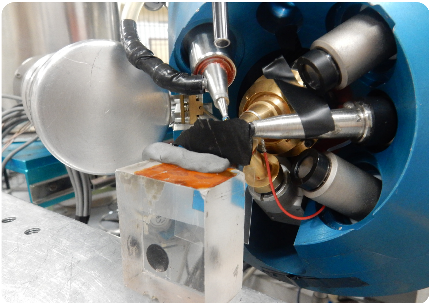
Particle-induced Gamma and X-ray emission spectroscopy testing on Whitby Jet (Photo by Sarah Steele)
