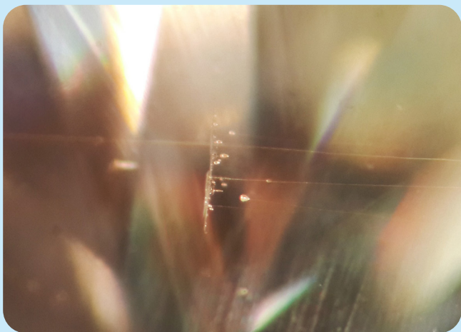
Figure 5: Pear shape gas bubbles in synthetic moissanite, some with stringers extending from the points of the pear shape gas bubbles.
