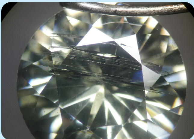
Figure 13: Sub parallel ribbon-like inclusion and stringers. Notice the doubling of the back facet edges is not visible through the table although the ribbons are almost parallel to the table. This proves that these ribbon-like inclusion can be formed in synthetic moissanite unrelated to its optic axis direction.
