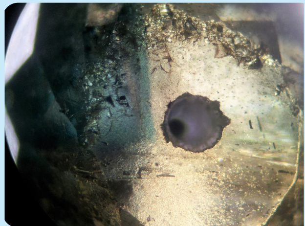
Figure 2: Angular green color zoning in synthetic moissanite.
