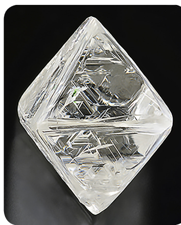
Figure 9. Image revealing the much steeper than 45° angles of octahedral diamond 'rough'. Photo by Robison McMurtry.
